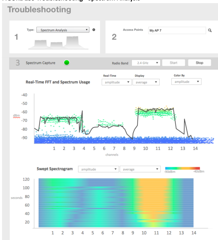
FIGURE 259 Troubleshooting - Spectrum Analysis
